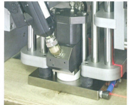
Injection head and cooling plate on the workpiece
